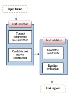
Fig. 3. Overall procedure of the proposed detection method
