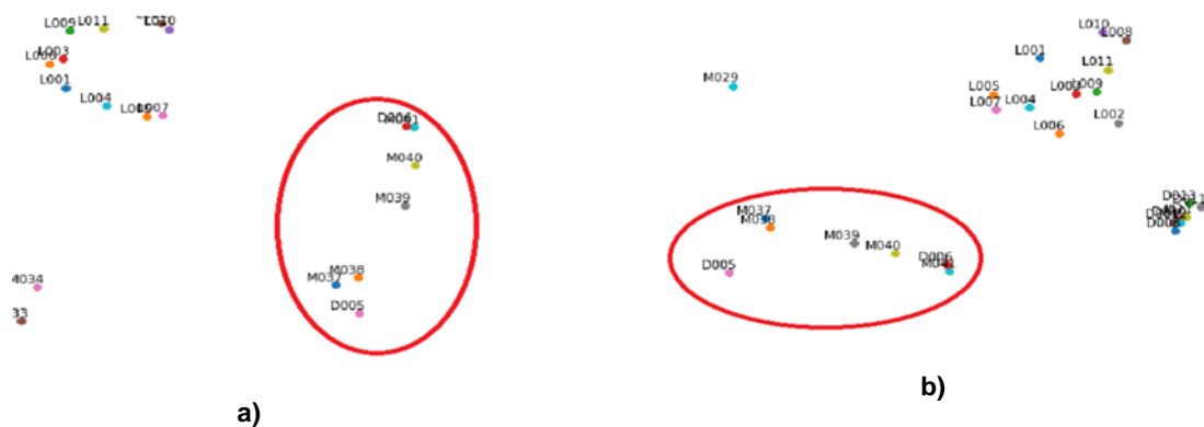
Fig. 4. Extract from the t-SNE plot of the activity of sensors from the CASAS Kyoto-20 dataset [11], using 600 seconds as the interval and time decay factor weight x^t for x=0.9 and t being the time gap in multiples of 15 sec, showing the contextual proximity of the motion sensors close to the toilet (M038 to M041) and door sensor D005
