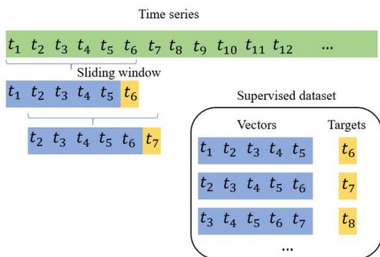
**Fig. 4.** Illustration of converting a time series to a supervised dataset. Source: Own elaboration
