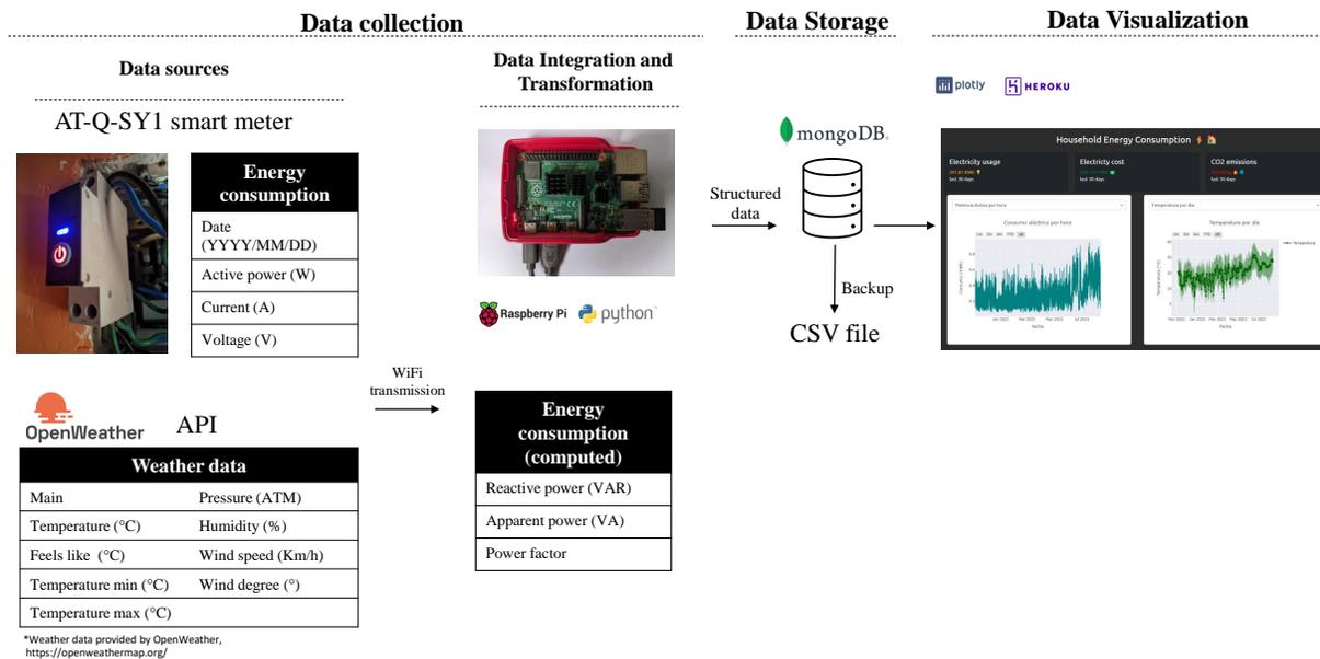
Fig. 2. Overall system diagram. Source: Own elaboration
