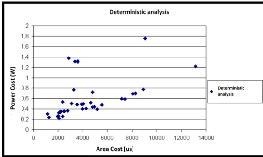
**Fig. 5.** Trade-off curve between area cost and power consumption cost for possible system implementations (Deterministic Analysis)
