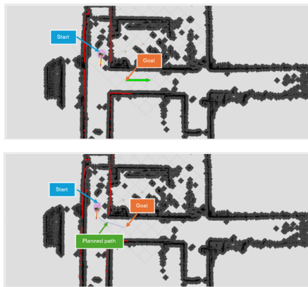
Fig. 4. RViz visualization of the navigation test in the T-shaped corridor. The upper image shows the goal pose definition, including the desired final position and orientation. The lower image shows the planned path and the initial execution of the trajectory-following stage
