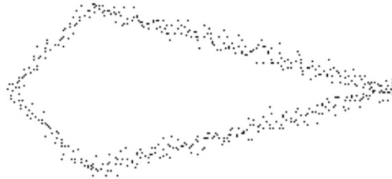
Fig. 3. An example of a Gaussian noise corrupted quadrilateral shape having \alpha = 50 , \beta = 0.25 , \mu = 0 and S = 4
