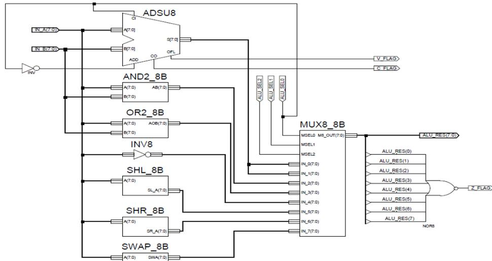
Fig. 7. Arithmetic and Logical Unit schematic diagram
