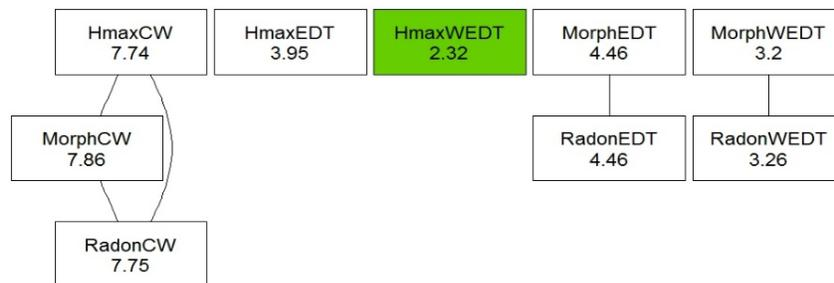
**Fig. 9.** Friedman test with the Bergmann and Hommel *post hoc* correction for the nine algorithms tested. Groups of methods that are not significantly different appear as connected nodes
